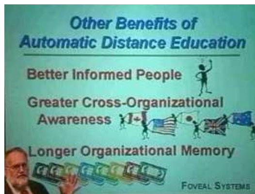
Figure 5. A Slide Camera sees gestures in front of the screen that a scan converter misses.
