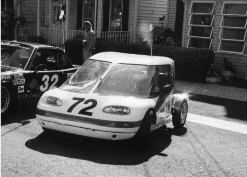
Figure 31 – ‘Sungo’ improves each year. This time it featured Horizon batteries, a BADICHEQ battery management system, and a spare battery pack that is the moral equivalent of a spare can of fuel in the trunk.
