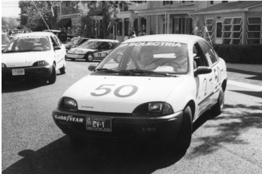
Figure 26 — This 'Solectria Force' ran on Horizon advanced lead-acid batteries. It achieved 138 Watt-hours per mile. It was also awarded the Best Sedan using Lead-Acid Batteries prize.
