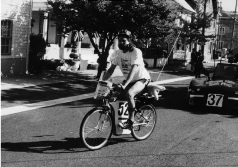
Figure 40 – ‘Electrobike’ may not look special until you notice the large rear wheel hub motor and the batteries mounted on the frame between the wheels.
