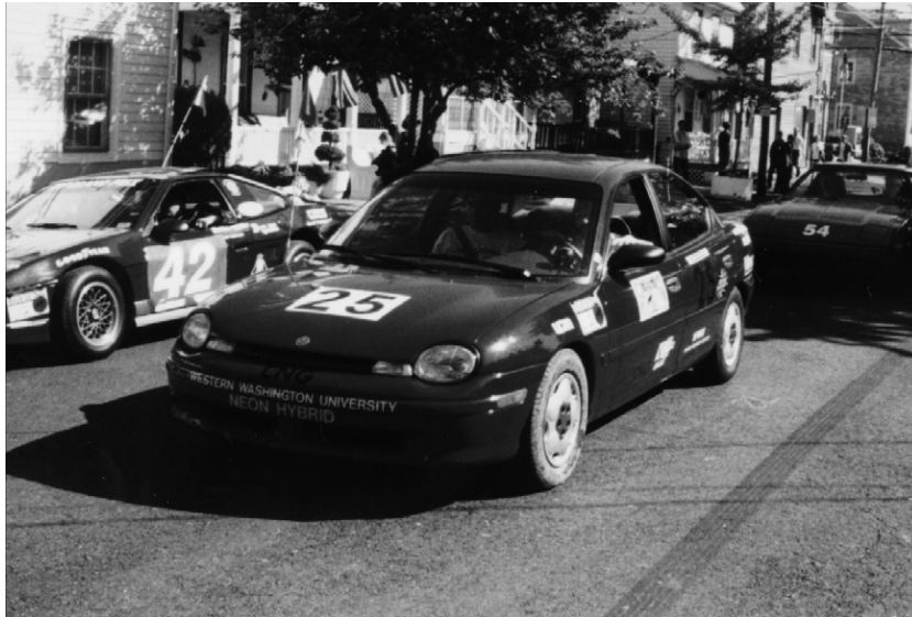
Figure 8 – 'Viking 25', a parallel hybrid that uses CNG as its fuel, was so clean that it met the California Ultra-Low Emission Vehicle (ULEV) standard.
