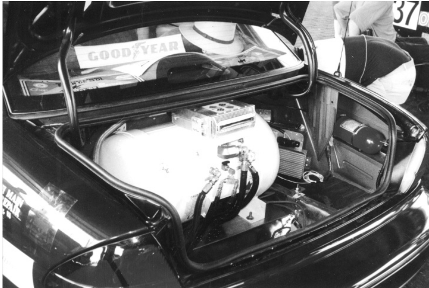
Figure 17 – Finding room for all the pieces of a hybrid conversion can be a bit of a challenge. Here the tank for the compressed gas used as a fuel takes up much of the trunk space. The horizontal slot on top of the tank is for a MagnaCharge padel.
