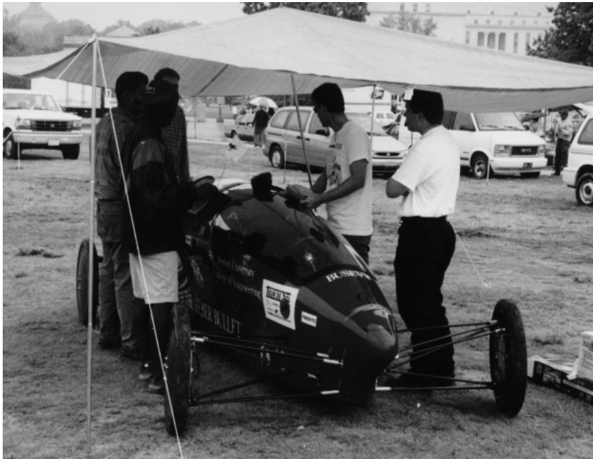
Figure 52 — The two people in Boston University's 'Silber Bullet' ride back-to-back, so as to keep the body narrow and aerodynamic.
