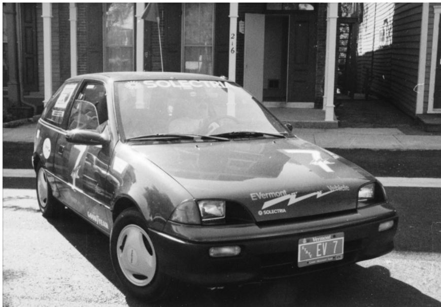
Figure 14 — The 'Nordick Challenger' is a 1994 Solectria Force that has seen 20,000 miles of Vermont summers and winters. A fuel-burning heater keeps the passengers warm in the sub-zero weather on only 3 gallons of kerosene a winter.
