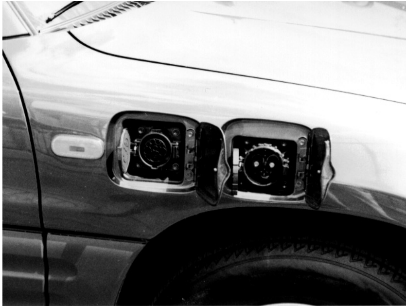
Figure 16 — Toyota's 'RAV4-EV' has two charging plugs. One is for an external fast charger capable of delivering high current. The other is to provide AC current for the on-board opportunity charger.
