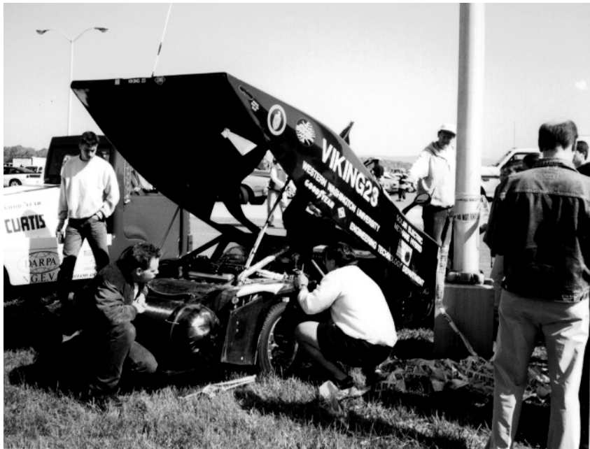
Figure 7 — 'Viking 23' opened up. The CNG tank strapped behind the rear wheels is made entirely of composite materials.
