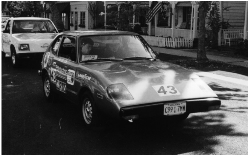
Figure 2 — The ‘KA1000’ has a long and checkered history leading to the NESEA Tour. It started as a Honda Civic, but the “nose job” changes its appearance and adds room for batteries.
