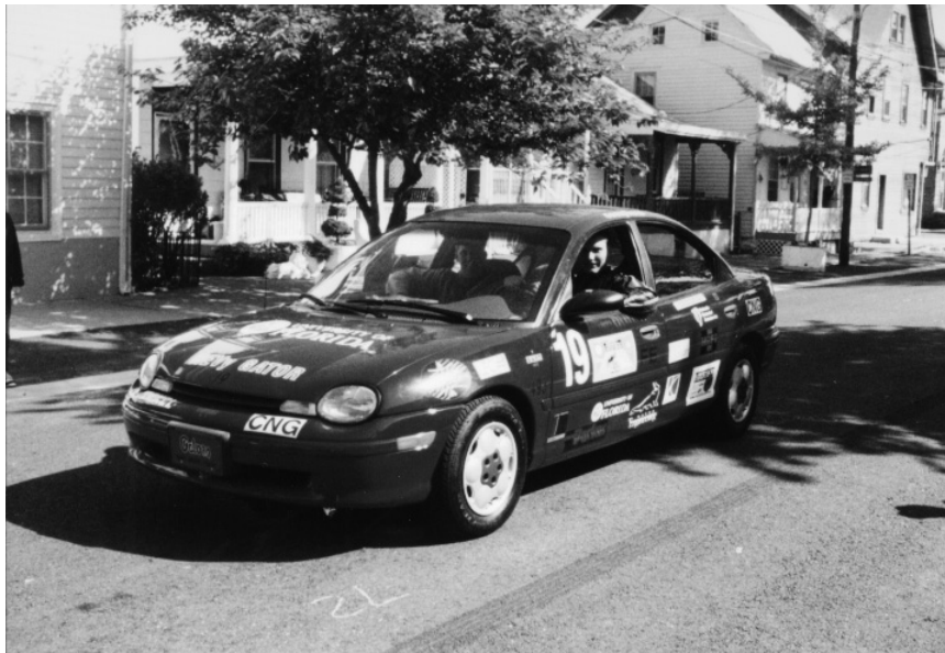
Figure 3 — 'HEV-GATOR' from the University of Florida in Gainesville is a series hybrid electric. Although the engine is still in the front, an electric motor now drives the rear wheels.
