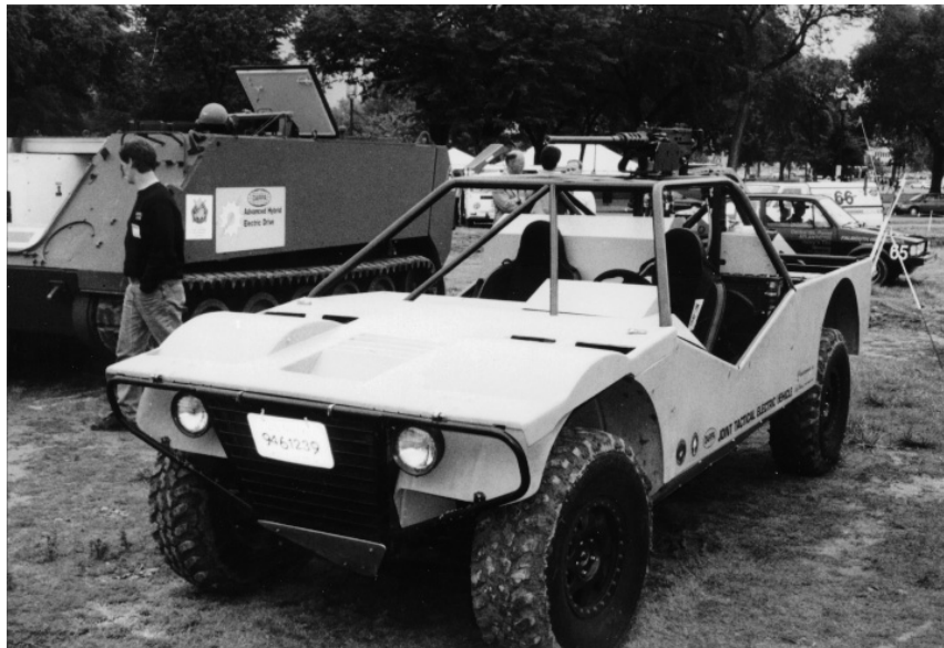
Figure 49 — The US military is studying the possibility of using EVs because of their low noise, heat, and exhaust signatures. This Joint Tactical Electric Vehicle is the result of such a study. And yes, that is an armored hybrid EV personal carrier in the background.
