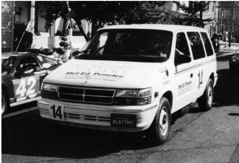
Figure 1 — This Chrysler 'TEVan' is based on a Dodge Caravan. It carries about 60 kiloWatt-hours of NiCad batteries to drive a GE shunt-wound motor.
