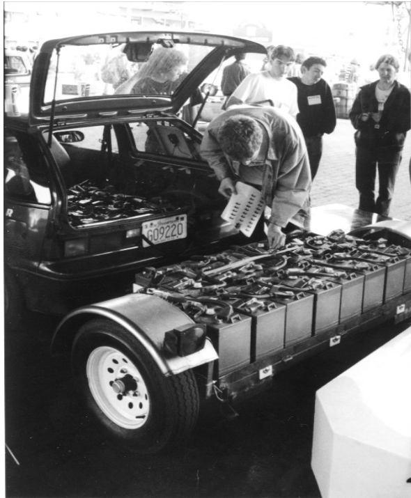
Figure 39 – ‘George the Geo’ has both its internal and trailer battery packs open for inspection. The pack in the trailer was used to let the larger internal pack “rest” a bit and recover some of its capacity. Switching back and forth proved quite effective in obtaining extra range. ‘Sungo’ (72) also used this strategy.
