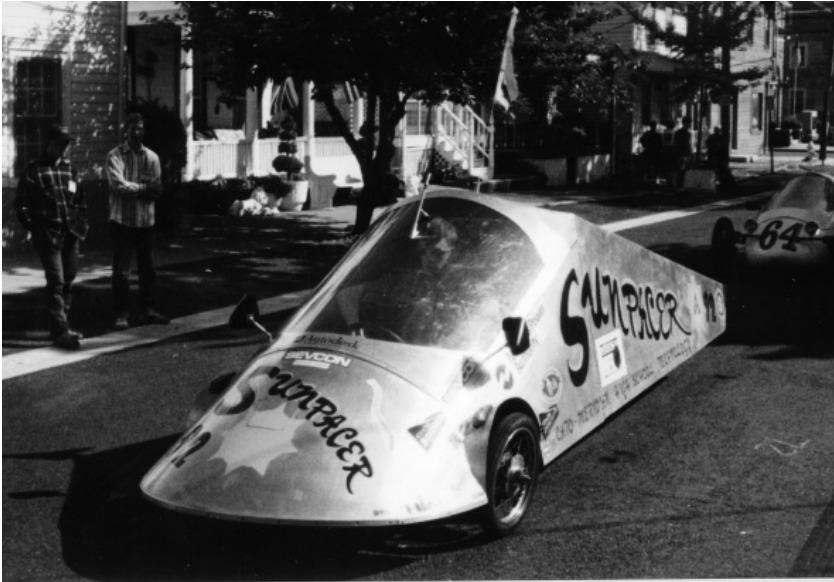
Figure 53 — ‘Sunpacer’ from Cato-Meridian High School in New York turned in an impressive efficiency of 82 Watt-hours per mile, second only to the much lighter ‘Twike’.
