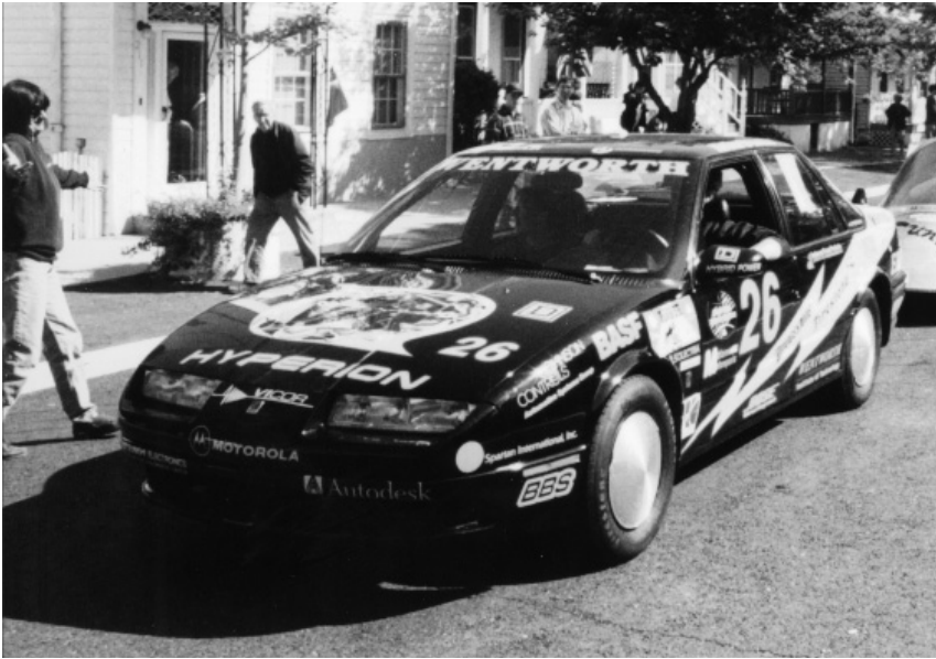
Figure 6 – ‘Hyperion’ is a parallel hybrid, constructed from a Saturn SL2. It now burns E-85, a mixture of 85% Ethanol and 15% gasoline and the exhaust smells a bit like moonshine.
