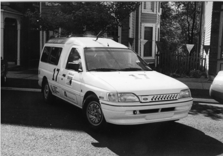
Figure 42 — Based on a European delivery van, the Ford 'Ecostar' uses Sodium-Sulfur batteries capable of delivering well over 100 miles per charge.
