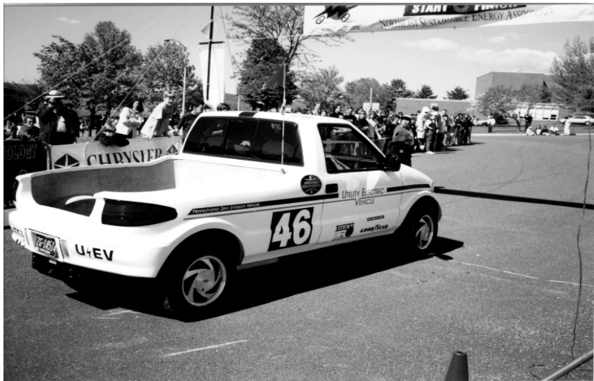
Figure 45 — The 'Utility EV' is a proof-of-concept project of the PETC. It is built almost entirely out of composite materials and so is very light and maneuverable.
