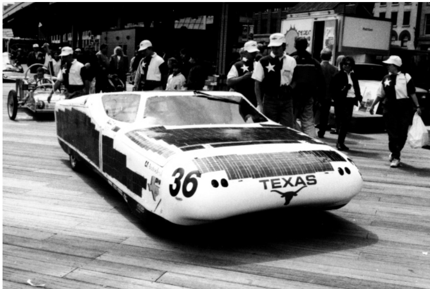
Figure 9 —'Texas Native Sun II' and team at South Street Seaport in New York City. The solar cells can collect up to a kiloWatt of sun-generated electricity.
