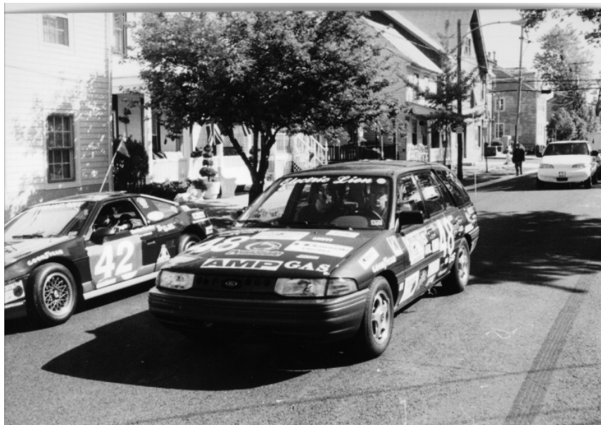
Figure 27 — The 'Electric Lion', a series hybrid from Penn State University, burns reformulated gasoline. It features separate electric motors driving each front wheel. Done properly, such an arrangement should make the car much easier to handle.
