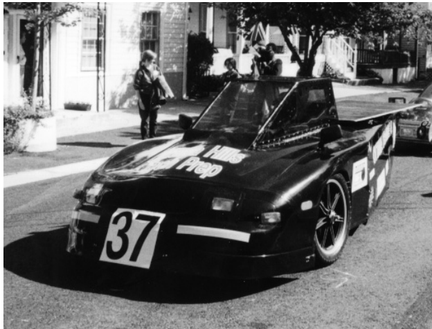
Figure 25 — 'Ottawa Orange IV' leaving Chesapeake City. The black body is a light, plastic faring over a box-tubing frame.
