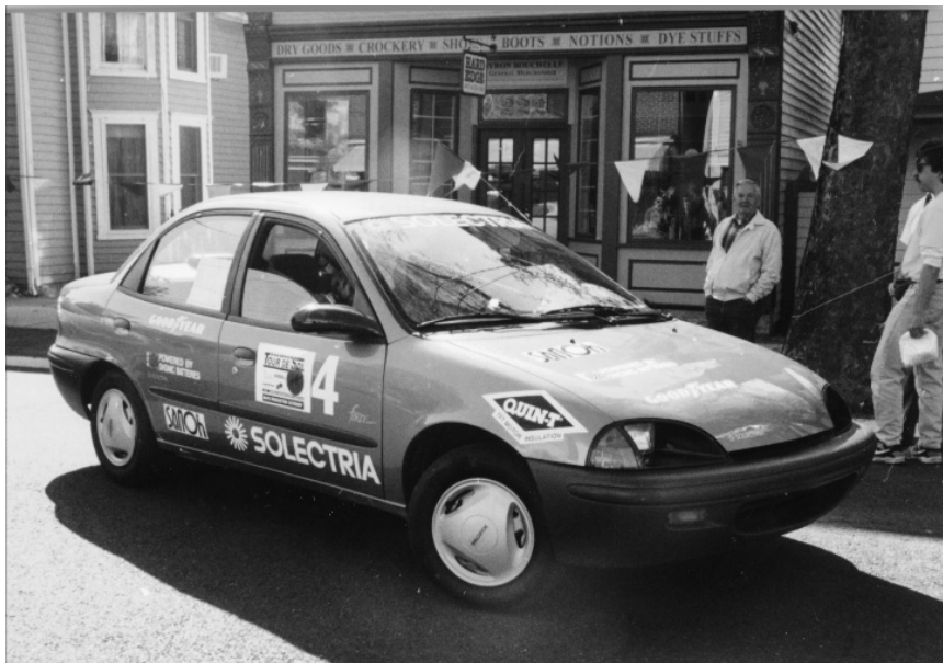
Figure 46 — This 'Solectria Force NMH' went over 240 miles on a single charge of its Nickel Metal Hydride batteries. It also delivered the equivalent of 60 miles per gallon during an urban driving-cycle test.
