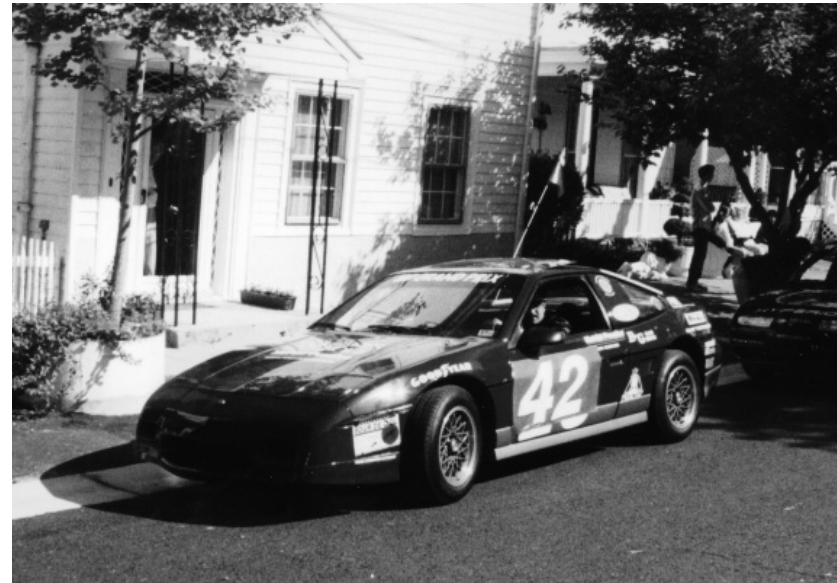
Figure 34 — The 'Golden Gear Special' is another high school project, based on a Pontiac Fiero. It has particularly large batteries which brings its curb weight to 3600 pounds.
